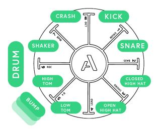
Drums are velocity-sensitive and will respond to different intensities of tapping, similar to how a traditional drum changes its tone and volume by hitting it harder or softer. The sounds also respond to how long your finger stays on each pad. Try holding your finger on a cymbal to cut it short, or tap and release quickly on a tom to hear a long decay.
